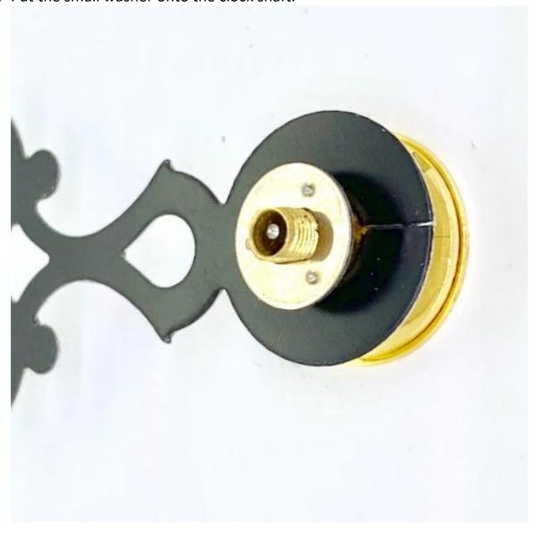
3. Put on the hour and minute hand as well as the top nut
